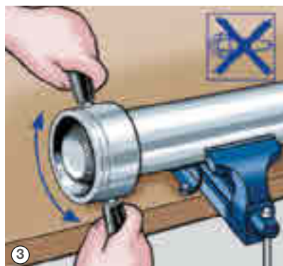
3 De-burr pipe internally and externally.
