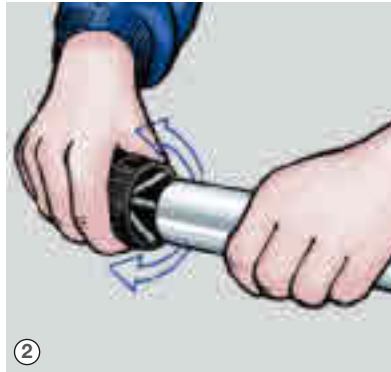
② De-burr pipe internally and externally.
