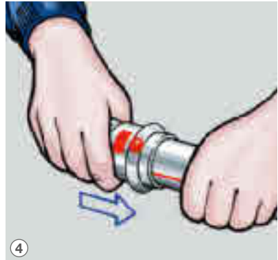
④ Slide the press connector onto the pipe as far as the stop.
