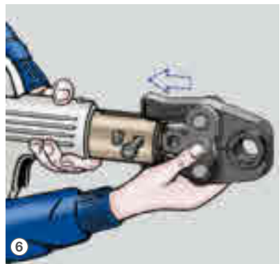
⑥ Place press jaw onto the press tool. Push in the retaining pin until it snaps into place.
