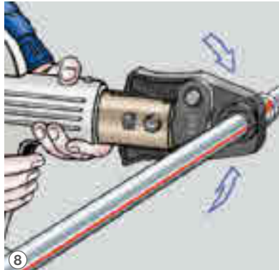
Check the insertion depth and start pressing.
