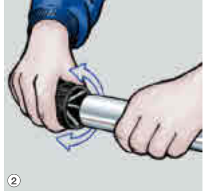
② De-burr pipe internally and externally.
