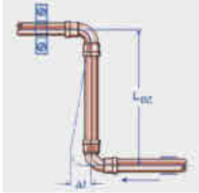
Fig. D—37 Z expansion compensating bend with XL-connector
