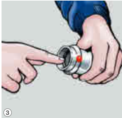
③ Check the sealing element is seated correctly.
