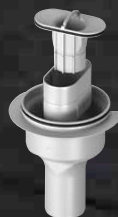
vertical model for construction heights from 40 mm, drainage capacity: 0.9–1.1 l/s*, water seal level: 50 mm (fire protection pipe lead-in possible) Model 4982.94
