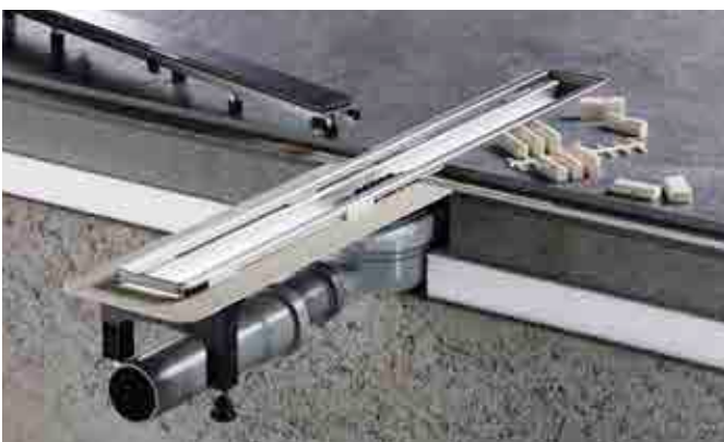
Parallel routing under the channel ensures that the connection pipe does not go through the screed.
