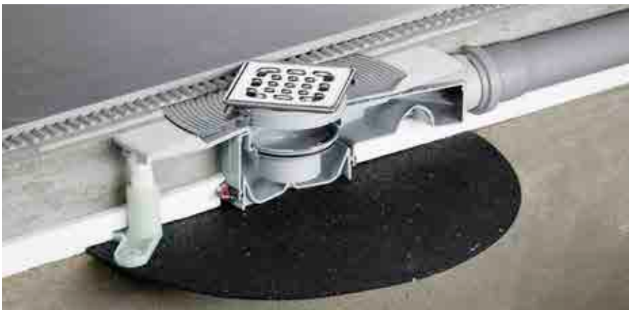
Advantix Top drain, backflow-proof by a water seal barrier with centred pass-through opening and lateral back-flow pockets.
